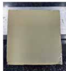
Glass/silver spray coating on Steel substrates for antibacterial character
